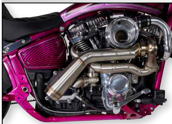
Trask's Tornado Turbo Kit looks fast sitting still. For good reason, the bolt-on upgrade provides a 40 percent to 50 percent boost in power.
