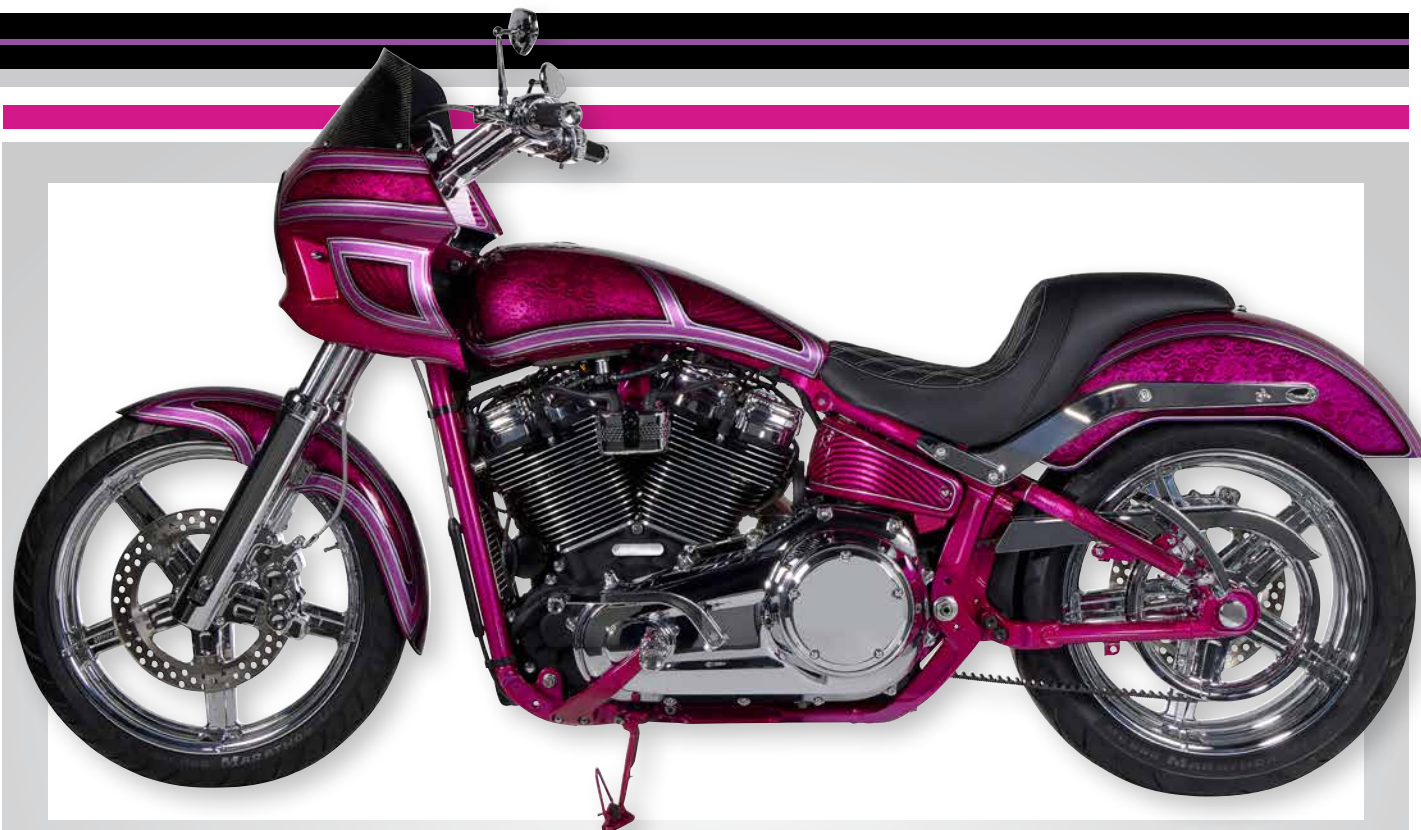
Trask's Tornado Turbo Kit looks fast sitting still. For good reason, the bolt-on upgrade provides a 40 percent to 50 percent boost in power.
