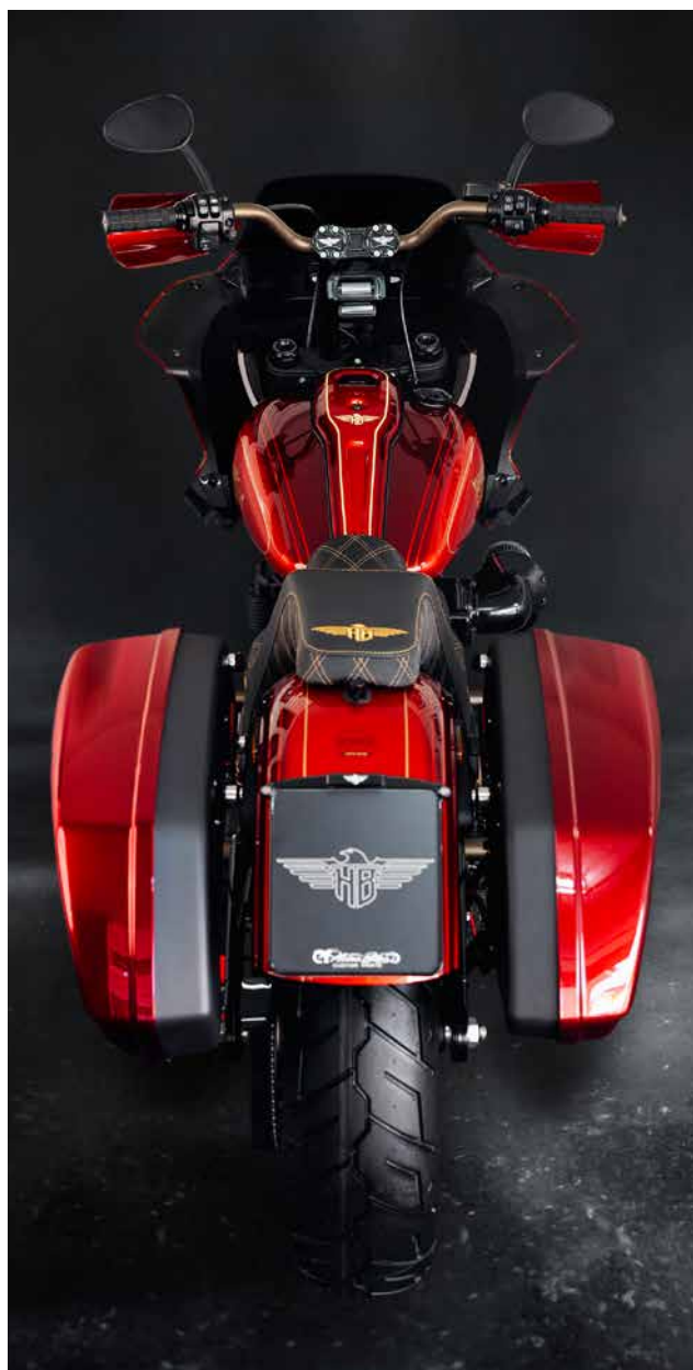
A HeinzBikes All-in-One NANO License Plate Holder anchors the rear of the bike. It serves as a plate holder, rear turn signals and taillights. The holder comes in fitments for plates from 10 different countries.
