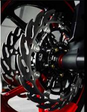
Moto-Master's Flame Series discs are available in both floating and fixed designs for many models. The unique flame design looks great and offers optimal cooling to keep braking consistent and predictable.
