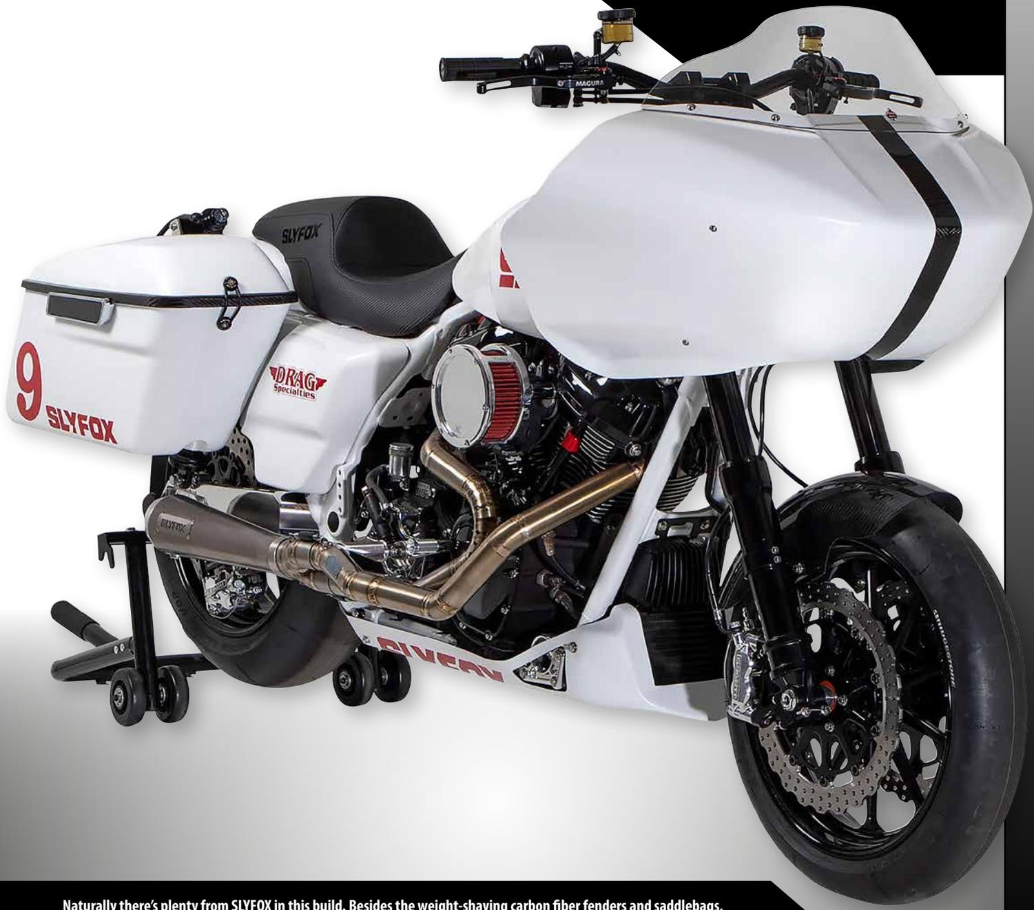
Naturally there's plenty from SLYFOX in this build. Besides the weight-shaving carbon fiber fenders and saddlebags, and a one-off carbon fiber fairing and bellypan, the wheels and brake rotors are SLYFOX, as well. The all-titanium exhaust is a collaboration between SLYFOX and Bassani.
