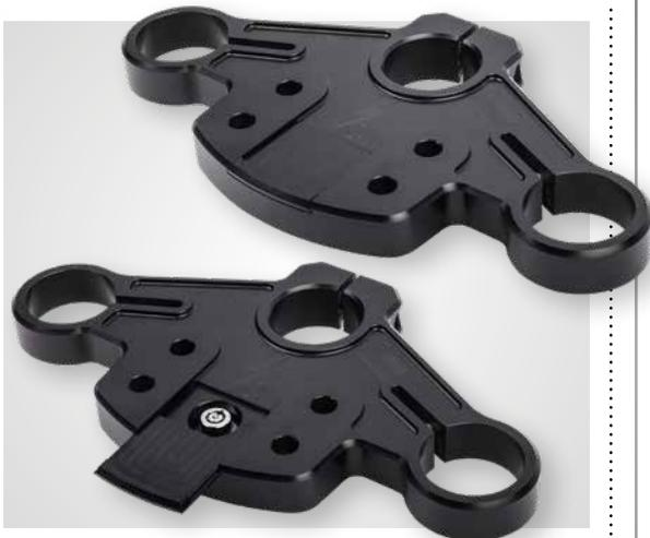
**With THRASHIN's new top triple for Road Glides, customers retain full fork-lock functionality – the lock sits behind a discreet spring-loaded cover. This top triple also provides two locations for riser installation for further fine tuning.**
