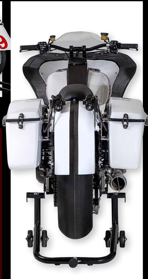
Beginning with an S&S Cycle 124-inch package and a complete Feuling valvetrain upgrade, the engine Alex Fox and the SLYFOX team spec'd out is race-ready. A Bridgestone Racing slick on a 6-inch wide SLYFOX Track-Pro wheel takes the power. It's covered with a SLYFOX carbon fiber fender and flanked with SLYFOX carbon fiber saddlebags and lids.
